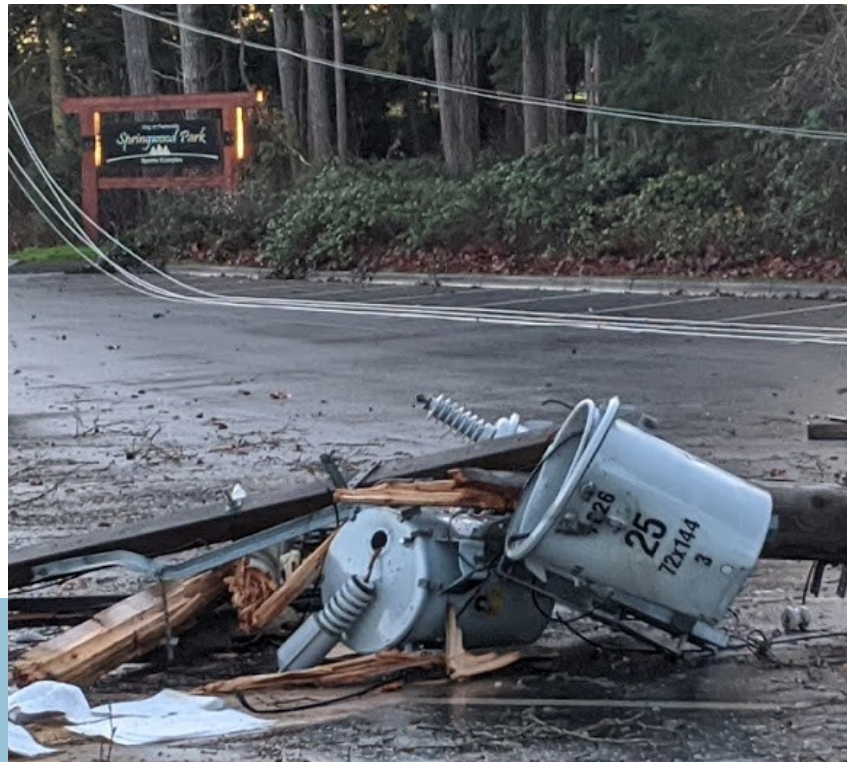
Power loss at Springwood Station due to a tree falling on power lines January 1, 2020
