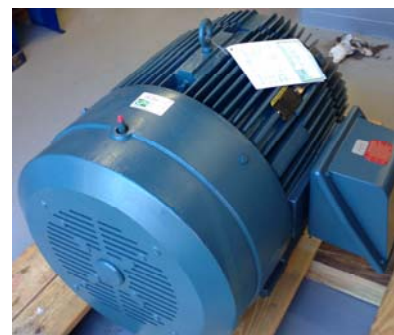
40HP pump/motor at Springwood
