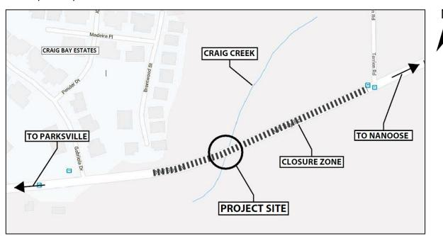
The Craig Creek culverts located on Northwest Bay Road just west of Terrien Road at City's boundary were identified for upgrade in 2017. Craig Creek, a salmon and trout stream, passes through the culverts under Northwest Bay Road. The culverts have presented problems of failing headwalls, elevated inlet and outlets restricting the movement of fish and capacity concerns during peak winter stream flows. This project falls under the scope of the Fisheries Act as well as the Species at Risk Act.
